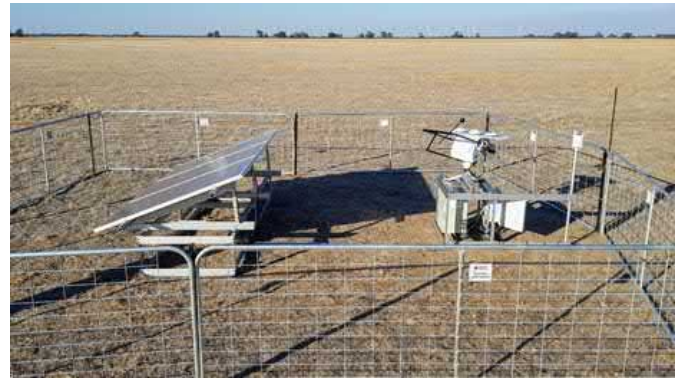
Fig 1: A typical solar-resource monitoring station
